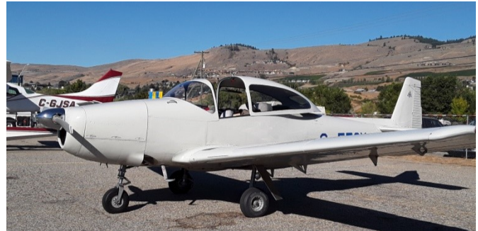
Grant Sherbeth's Navion C-FFGY The Ryan Navion is a single-engine, unpressurized, retractable gear, four-seat aircraft originally designed and built by North American Aviation in the 1940s
