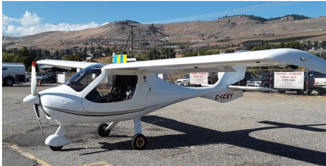
C-ICEY - Advanced Ultralight with Rotax engine - Flight Design CT2K. The Flight Design CT series is a family of high-wing, tricycle undercarriage, two seat, ultralight and light-sport aircraft produced by Flight Design (Flightdesign Vertrieb) of Germany.
