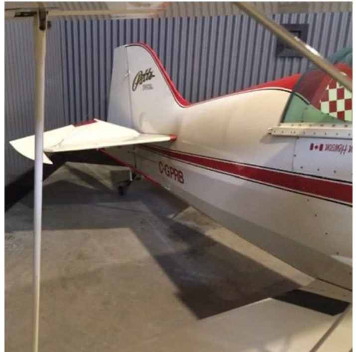
Elevator has large custom servo trim tab
