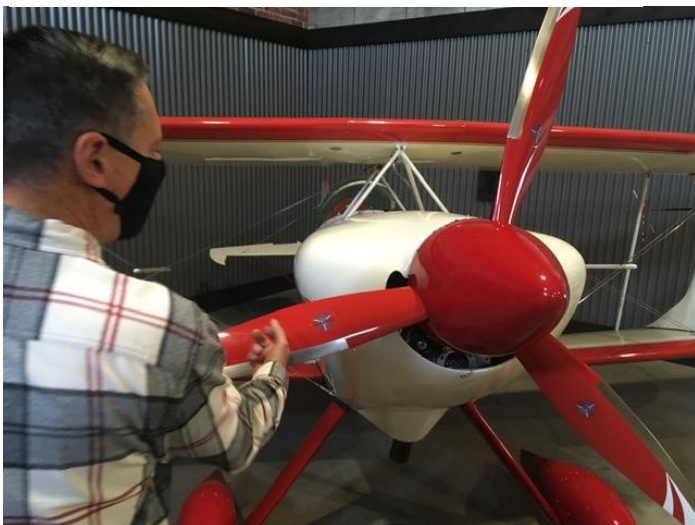
Ken pointing out the 3-bladed carbon prop
